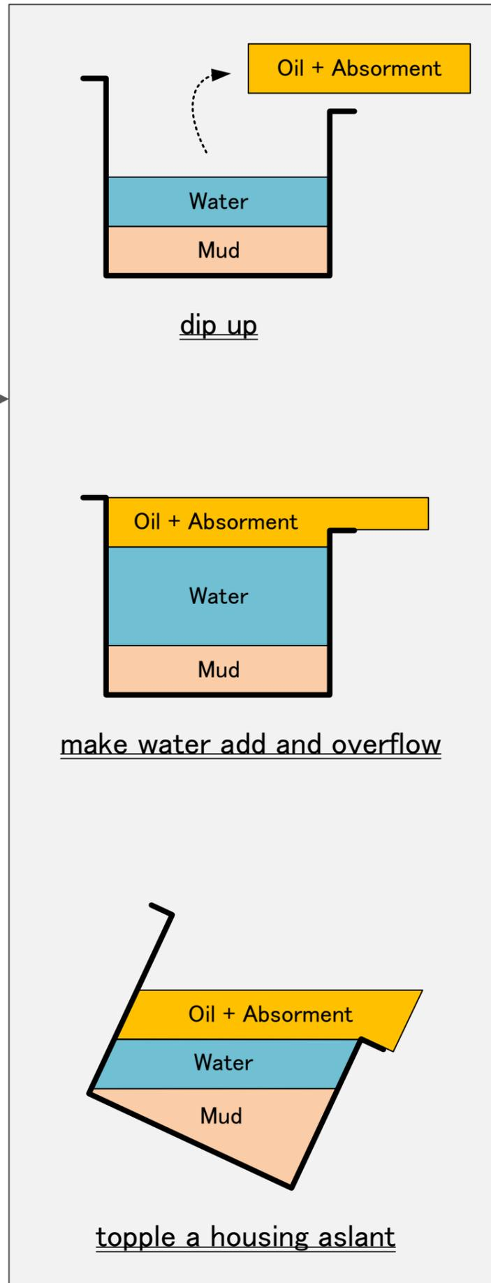
The work-operation flow in the case of processing the soil containing oil
